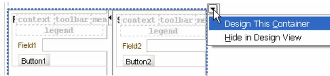
Selecting **Design This Container** opens an editor area that allows you to resize the component borders so that you could create a layout such as the following, where all components fit within the panels.
